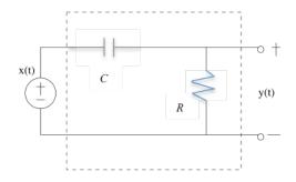
The initial voltage across the capacitor is 0V, and hence, the circuit is a linear time-invariant system.
